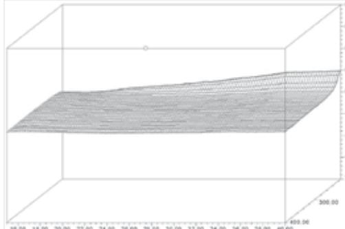
PDA gradient between 200-400 nm of Acetonitrile Vs. Water ULC/MS grade. Loading for 15 min. gradient 10-100% Acetonitrile in 20 min., hold 5 min. Column RP18, 3.5um; flow 1 ml/min.
