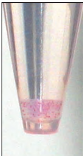
Visible Agarose Beads. Beads are easy to visualize, making it easier to avoid potential loss during washes and aspirations.
