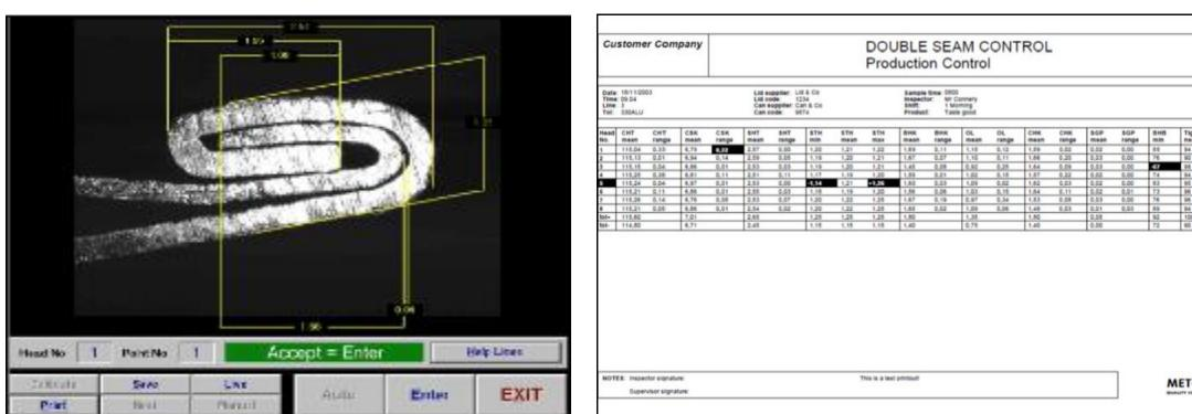
**A rating system evaluates all internal seam dimensions** and highlights critical errors.
